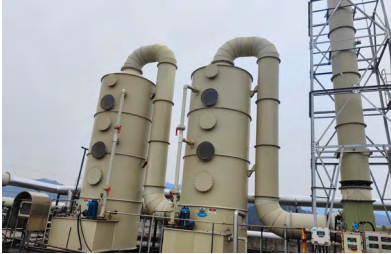
Tail gas absorption tower with multi-stage spray absorption, ensures a removal efficiency of over 95%.
